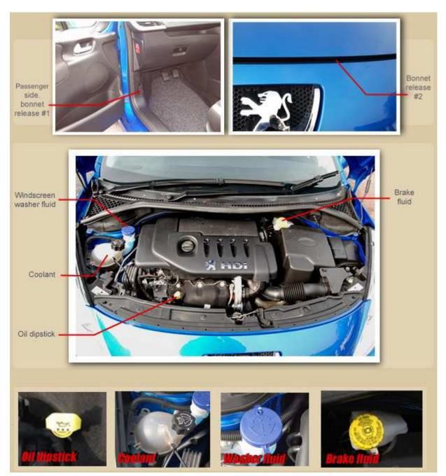
How to open the bonnet of a Peugeot 207 and identify whats underneath...
